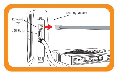
Wait 60 seconds for your modem to clear its memory completely. 4. Connect one end of the blue cable to the Ethernet port on your modem. Connect the other end to the blue port labeled "Internet" on the back of the Vonage Device.
